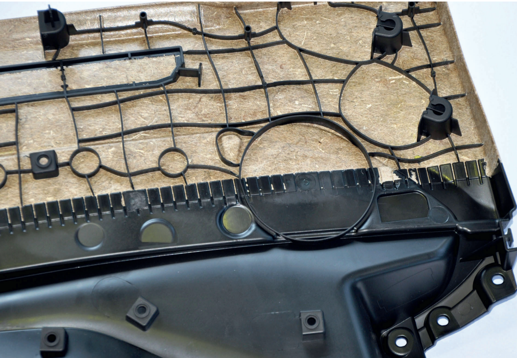
The B-side of the door trim manufactured by foam injection molding shows the reinforcing ribs behind the natural fiber mat and the molded-on map pocket at the bottom. © Frimo
