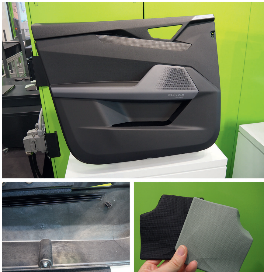
Fig. 4. Plastic, color and reproduction in a ceramic-coated mold produce a partial textile appearance (right). Various textures can be combined in one part (top), only the reverse side (left) shows the surface defects of foaming. © Hanser/C. Doriat
